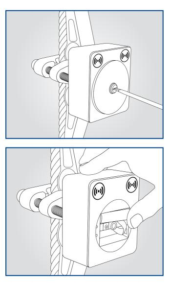
**IN A SAFE AREA ONLY**, remove the side cover of the BOLT using a flat blade screwdriver. Fit batteries and refit cover. The BOLT may be connected to the Straightpoint SW-HHP ATEX handheld, in hazardous areas, or to our range of load monitoring software that is not covered in this manual.
