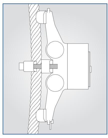
Note: It is important that the two bolts are tightened equally, if not it could show incorrect readings
