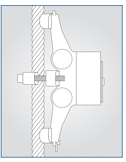
Make sure the bolts are torqued up equally, the torque rating is provided on the calibration certificate.
